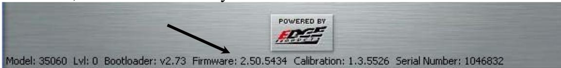
When your device is connected to Fusion, the Device Model, Level, Bootloader, Firmware, Calibration and Serial Number are all displayed at the bottom of the screen. These numbers will be useful to quickly view the state of your device, and whether or not it is currently programmed to a vehicle.
