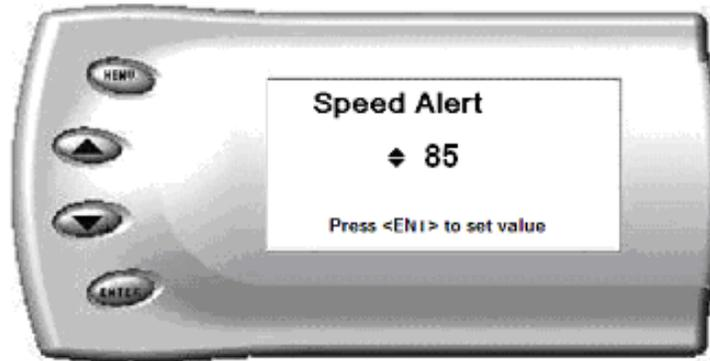
4. Press the [UP] and [DOWN] arrow keys until you have reached the desired value. Pressing [ENTER] will save the current alert value and return you to the Alerts screen. If you would like to change another parameter, select that parameter and repeat the steps.
