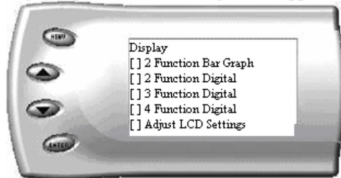
3. Select the desired viewing option by using the [UP] and [DOWN] arrows and pressing the [ENTER] key on the desired display type. Below are examples of the display options:
